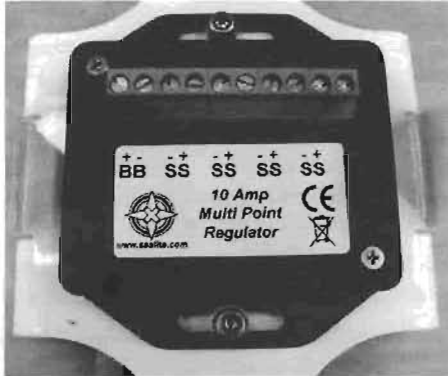
Use the label to ensure correct location of wires during assembly
